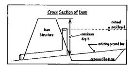
4. A cross-section of the dam (or embankment) indicating the maximum depth.
